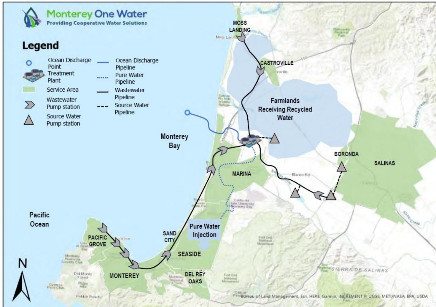
Figure B-1. Current Regional Map of Monterey One Water (M1W) Regional Treatment Plant (RTP) and Advanced Water Purification Facility (AWPF) Infrastructure Components
