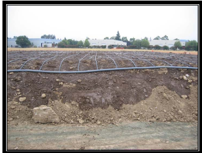
Figure 2 – Ex Situ soil pile showing wetting front.
