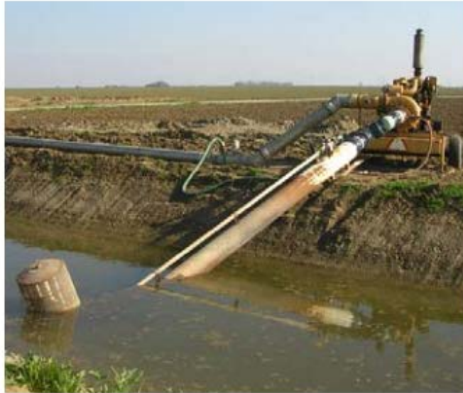
Figure 6. A rotary pump intake screen and diesel engine used for tailwater return. Photo: Lawrence J. Schwankl.
