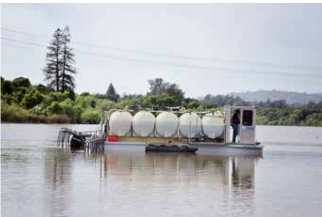
Photo 16 HAB Aquatic Solutions, LLC. barge dosing Pinto Lake with alum, April 2017. [Credit: Catherine Bosley, HAB Aquatic Solutions, LLC.]
