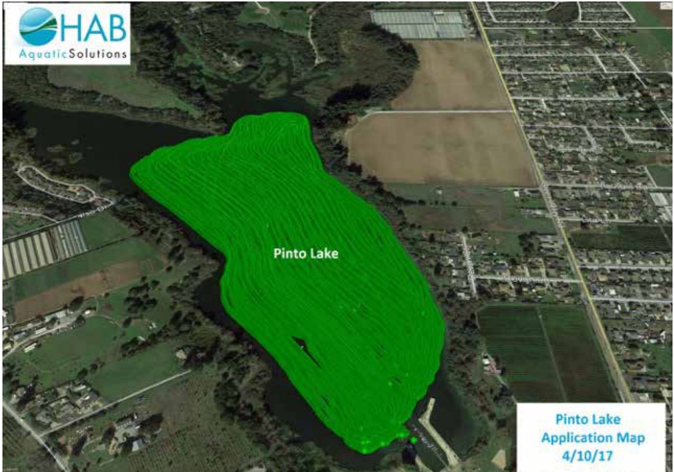
Figure 4 GPS printout of on barge tracking of the alum treatment, HAB Aquatic Solutions LLC.
