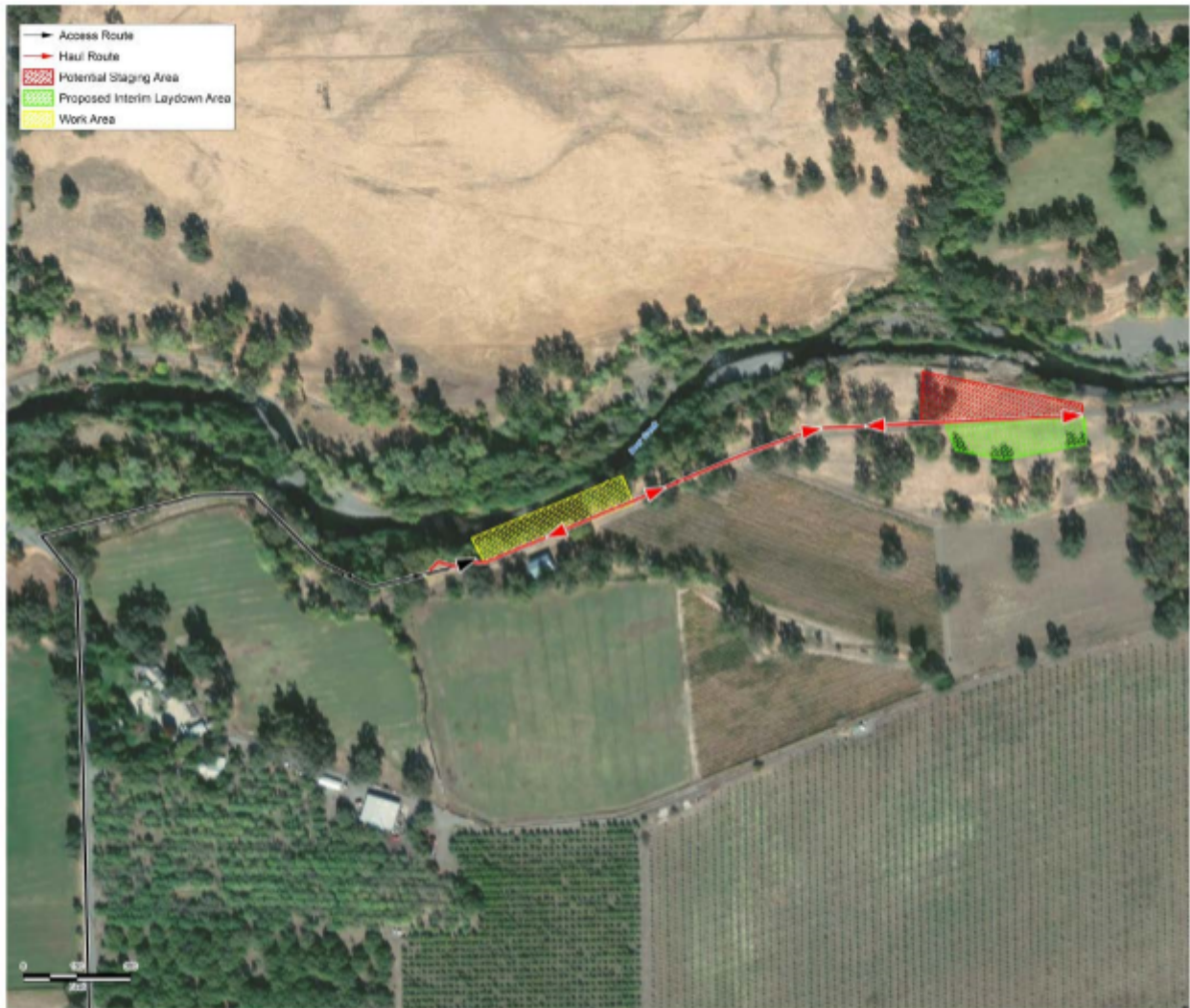
Figure 3: Proposed construction work area, staging and laydown areas, and haul and access routes for Deer Creek Levee Erosion Repair Project.
