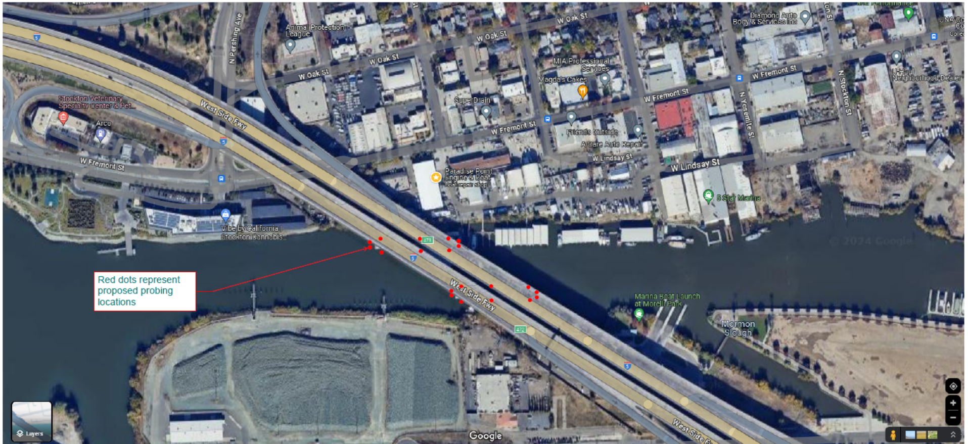
Figure 2: Project Probing Locations
