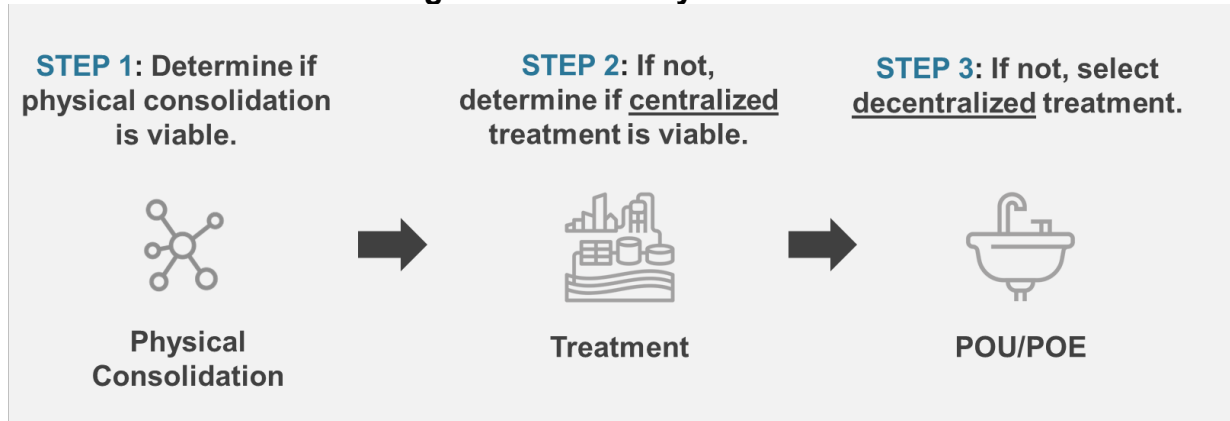
Figure 2: Proposed Updated Cost Assessment Model Long-Term Solution Selection Process for Failing Public Water Systems
