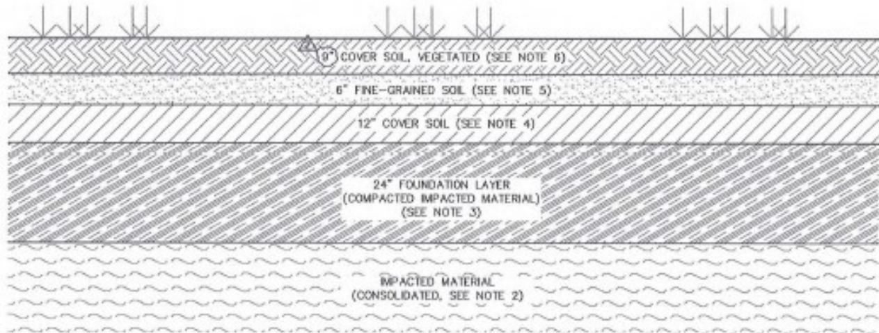
901 TYPICAL COVER SYSTEM DETAIL 8 NOT TO SCALE
