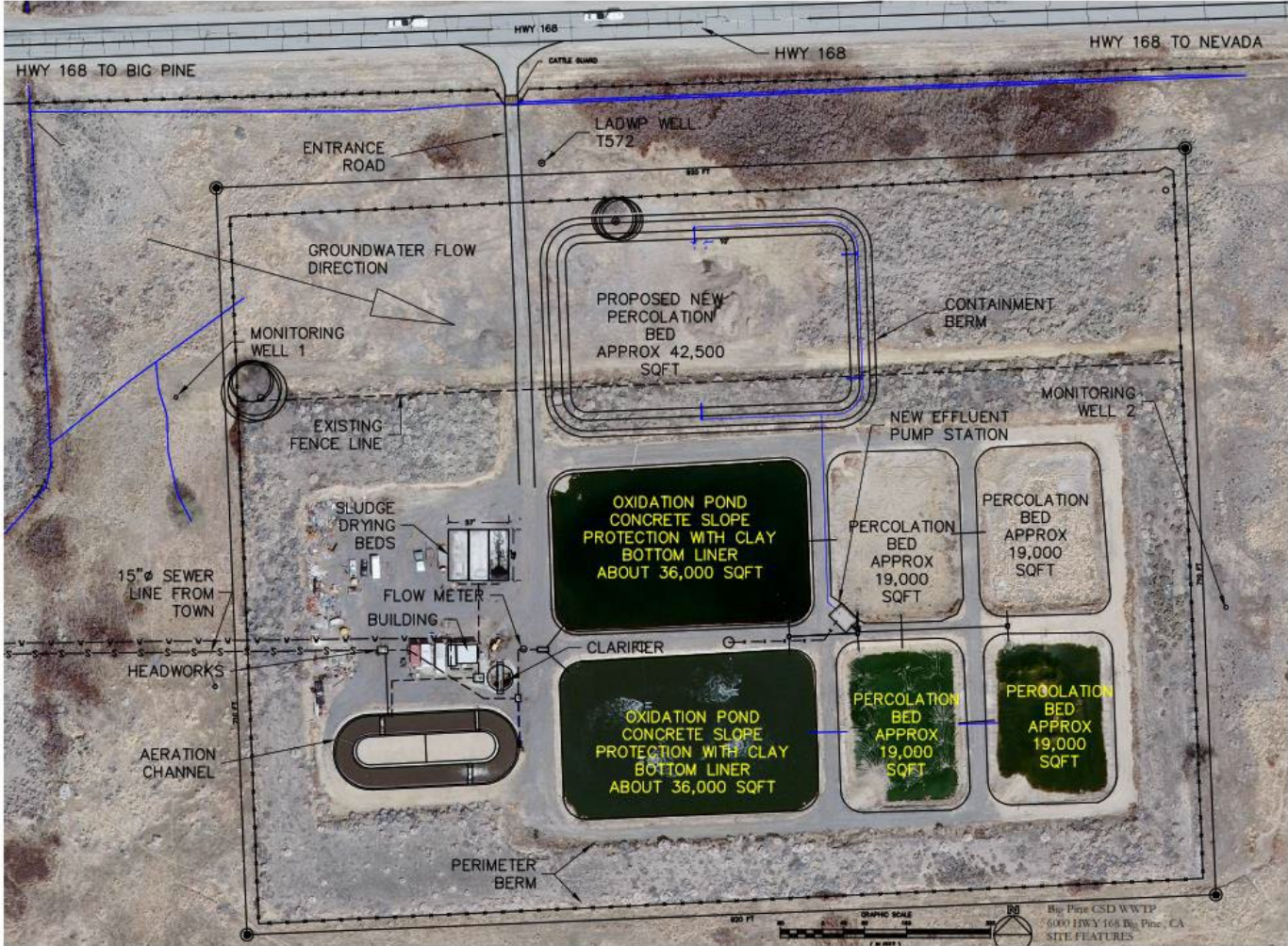
*Design drawing is from Big Pine CSD Report of Waste Discharge, Figure 3: Facility Map with Background Photo
