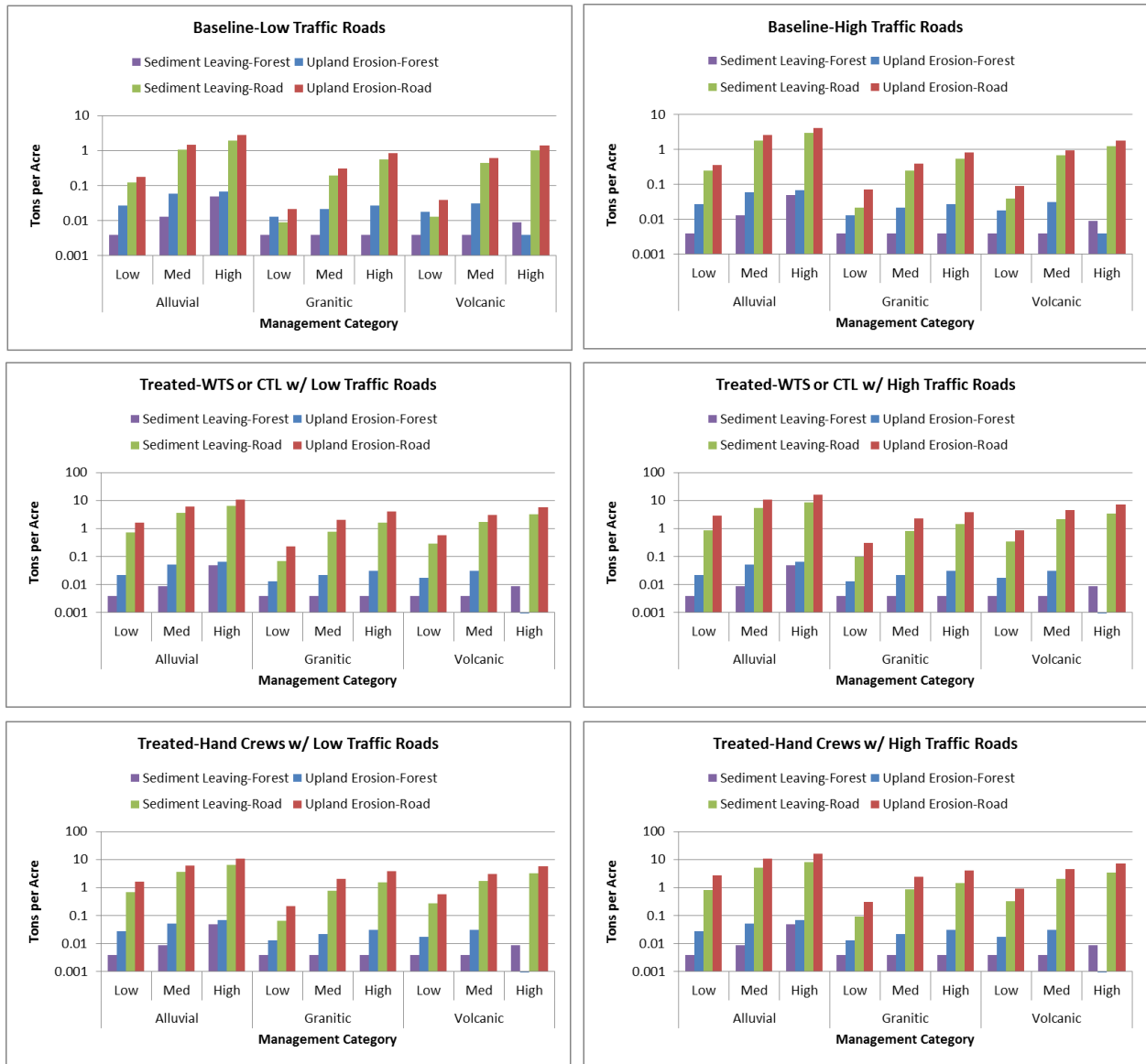
Figure 5-1. Unit area sediment loading on a log scale for treatments by management category with low and high traffic roads.
