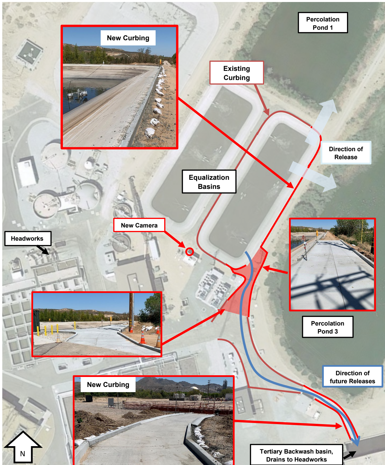
Figure 9.1 VVWRA Regional Plant - Overview of Inadvertent Release. Photo Courtesy of Google Earth 2018.
