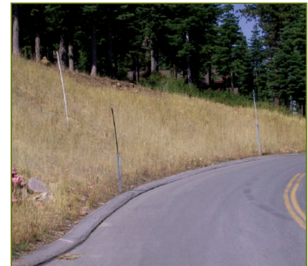
Contiguous slopes at Northstar Unit 7 in 2006 — hydroseeding treatment (left); full soil treatment (right).
