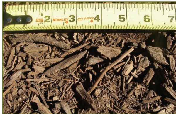
Coarse-textured compost blend – 50% coarse overs (3/8" – 3"), 50% fines (< 3/8")
