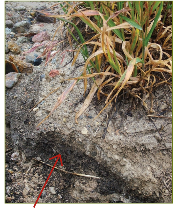
Buried topsoil layer revealed by gully on Sierra ski run.
