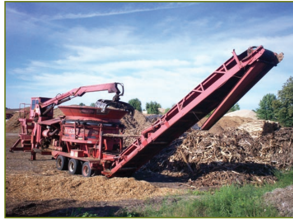
Tub grinders are used to grind stumps, root wads, and other large wood material that is too large for a chipper.
