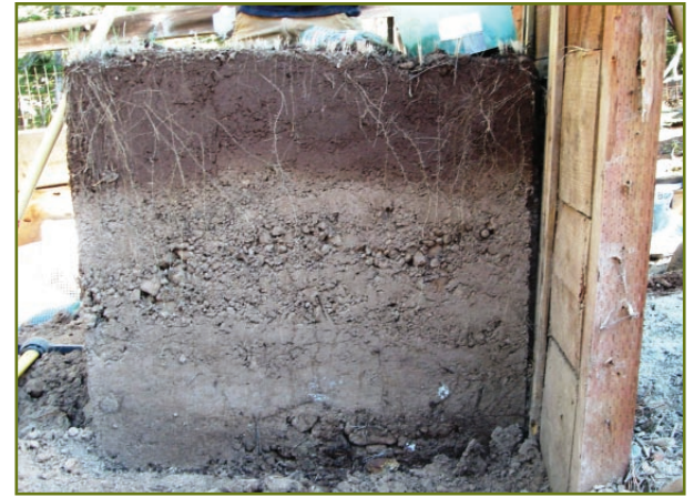
How deep are native plant roots? At a study site in Tahoma, California (Lake Tahoe), the roots of native perennial grasses extended to 46 inches deep in research boxes filled with uncompacted soil from nearby areas.
