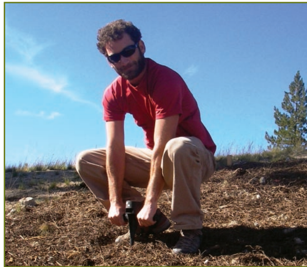
Measuring tilling depth with a cone penetrometer immediately after test plot construction.
