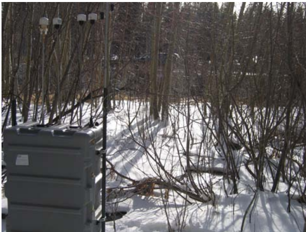
3 Figure 5. Four Deposition Boxes and UCD DRUM sampler at the Bourne Meadow site. 4 Top left: daytime upwind sampler 2; Top right: daytime downwind sampler 1 at 5 m away 5 from road, and RDI sampler; Bottom left: daytime downwind Sampler 3 at 30 m away 6 from the road; Bottom right: daytime downwind sampler 4 at 100 m away from road.
