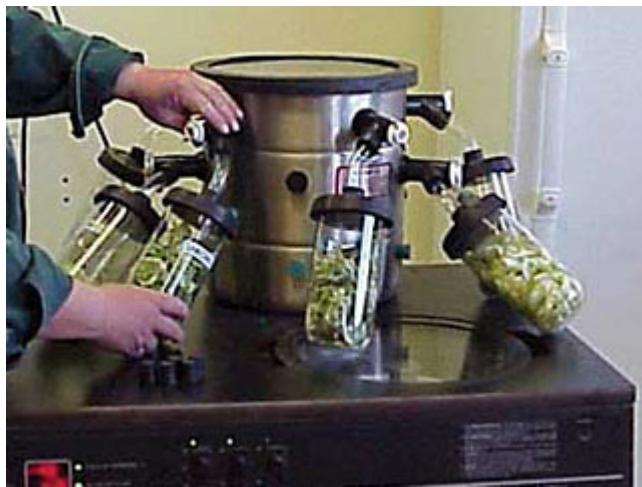
Lettuce samples are freeze-dried to prepare them for perchlorate analysis. Yuma Agricultural Center image.
