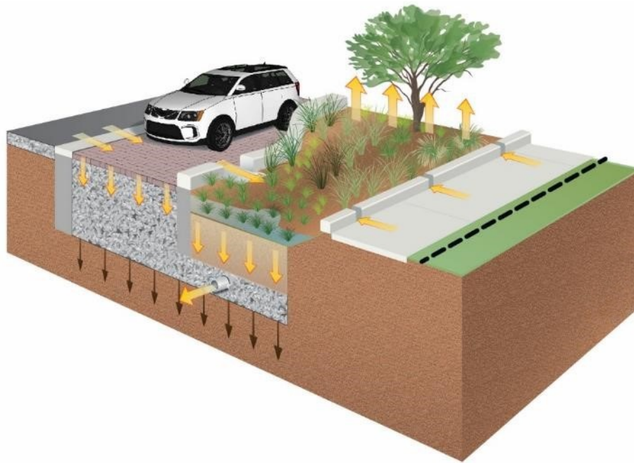
Figure 5-2 Conceptual Schematic of Green Street (arrows indicate water pathways)
