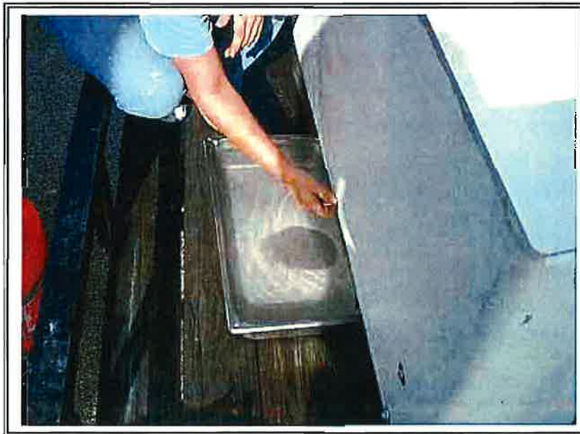
Photo No. 12: Sand in the Curb Inlet testing bed reservoir being washed into a container prior sieve analysis
