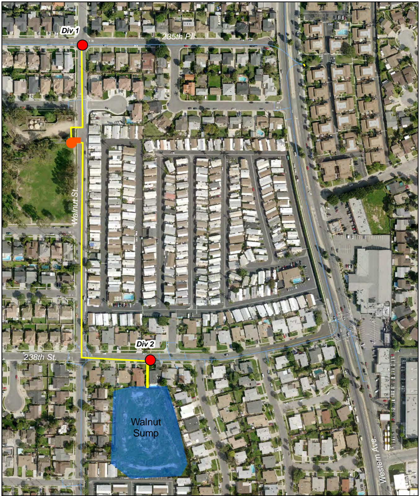
Figure 5.10 Conceptual Layout of Walnut Sump Aboveground Storage/Infiltration BMP Stormwater Recharge Project City of Torrance
