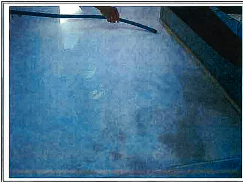
Photo No. 14: Sand left in lower tier of Skimmer Box test bed being washed into a container for sieve analysis
