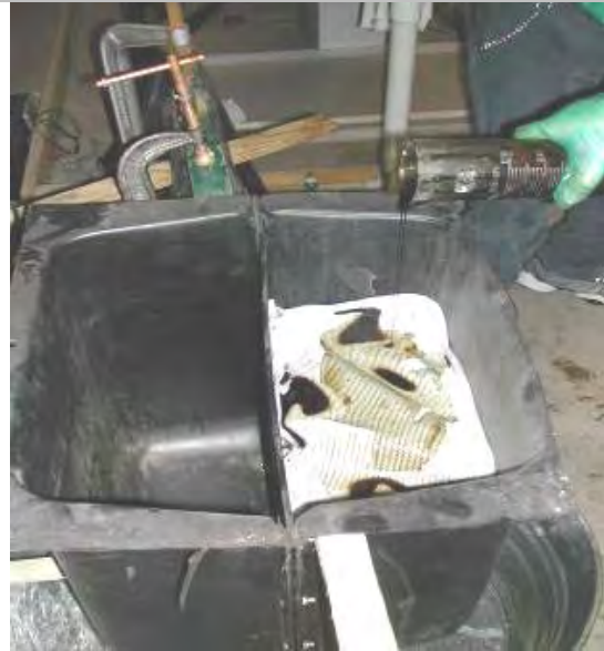
Pouring oil on HydroKleen
