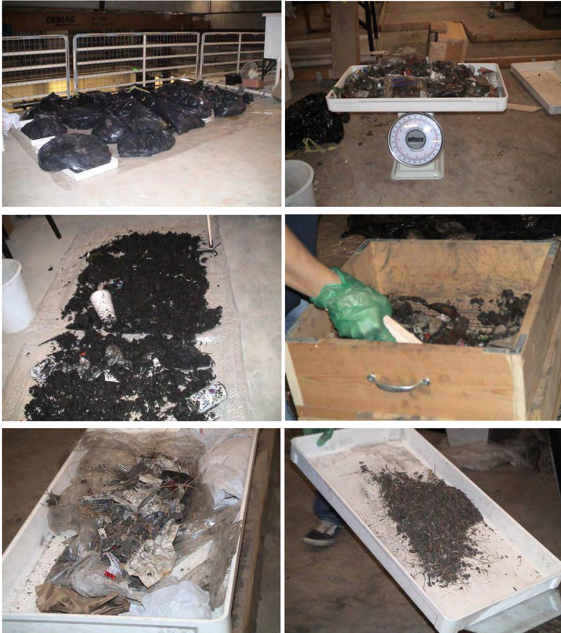
Figure 4-26. Photos of bulk solids screening process.
