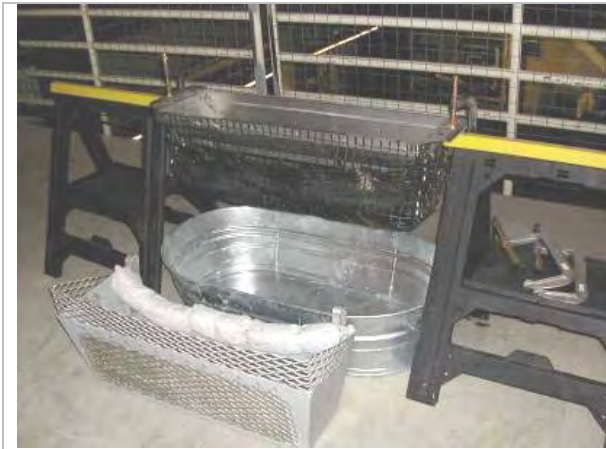
Laboratory set up for testing oil spill capture efficiency
