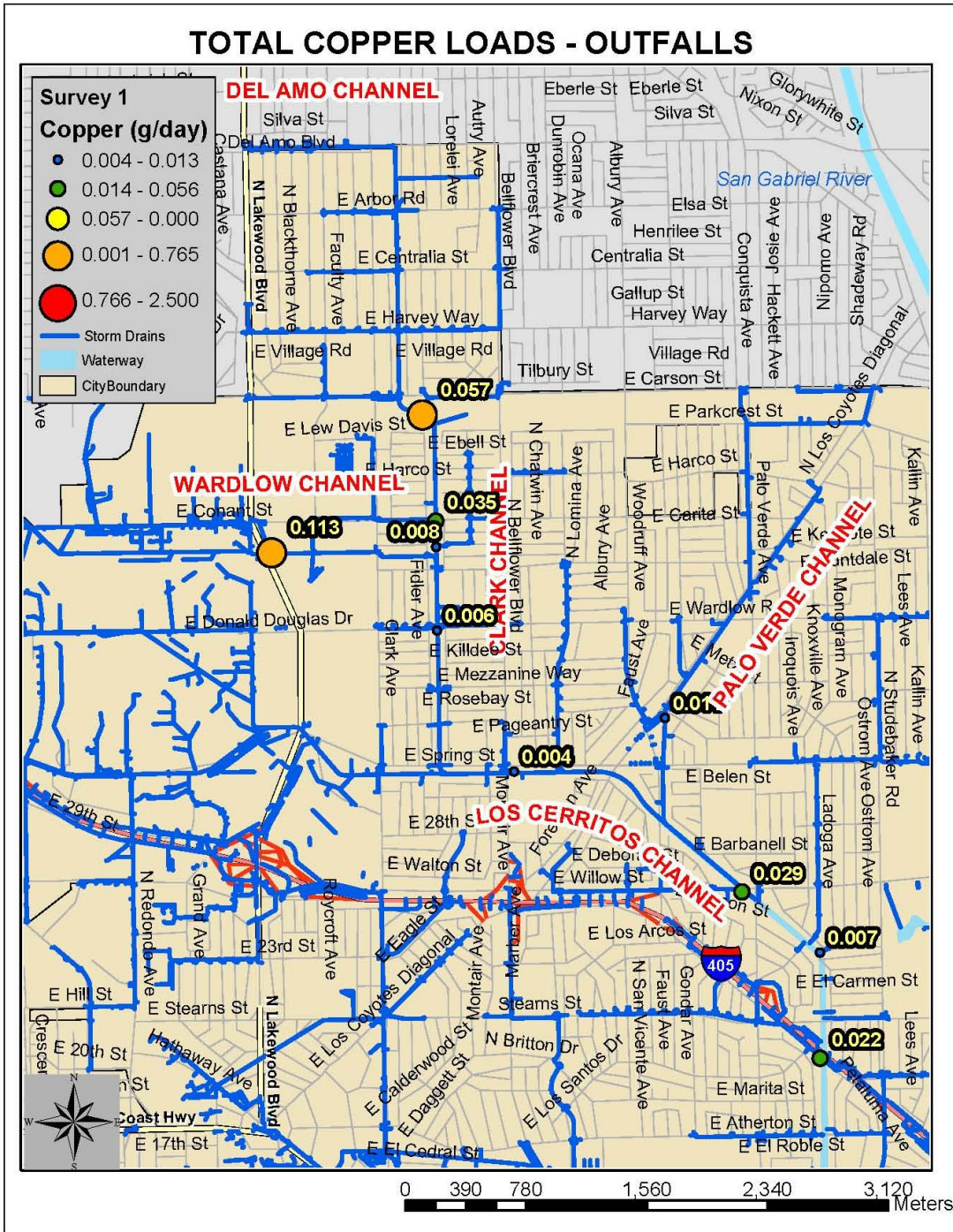
Figure A-37. Total Copper Loads Measured in Flowing Outfalls during Survey 1.
