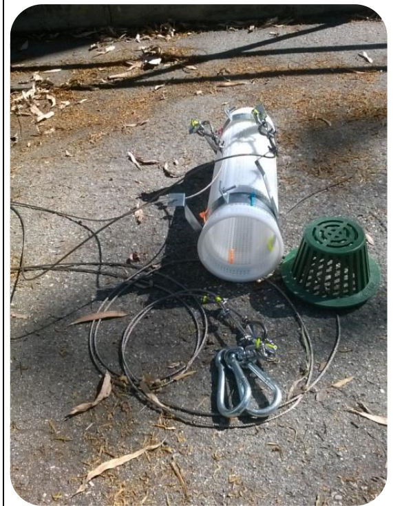
Storm-borne sediment sampling device used d at a catch basin
