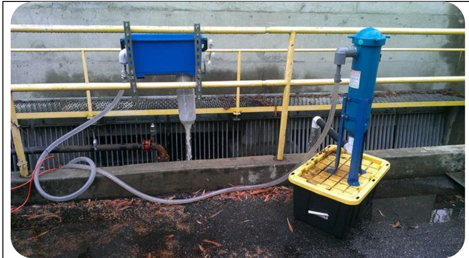
Two different filtration units designed to sample storm-borne sediment from a well
