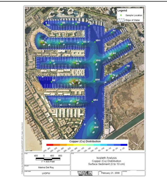
Figure 13. Distribution of Total Copper in Surface Sediment in Marina del Rey Harbor (Weston, 2008)
