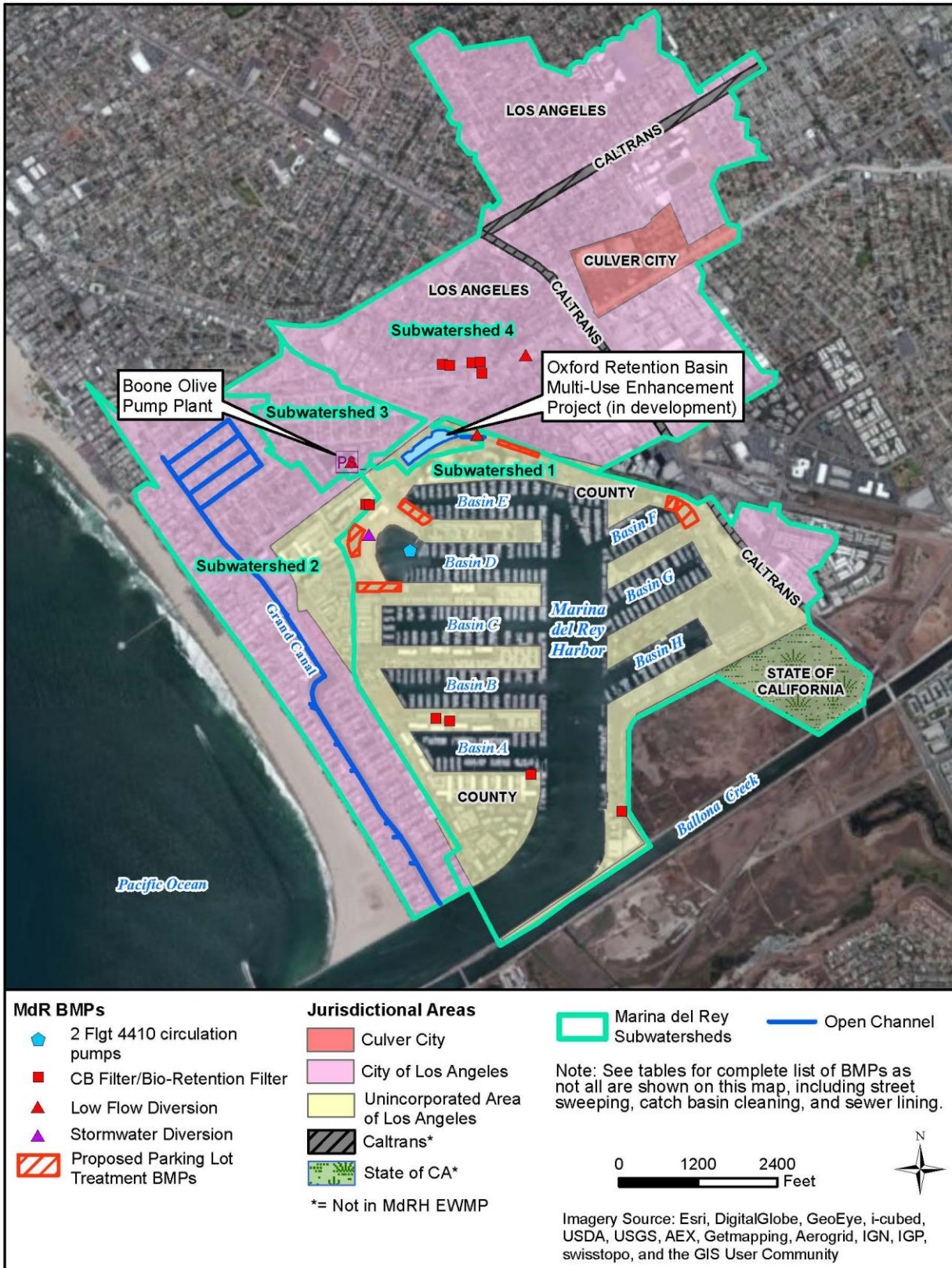
Figure 12. Existing Structural Control Measures within MdrH Boundaries
