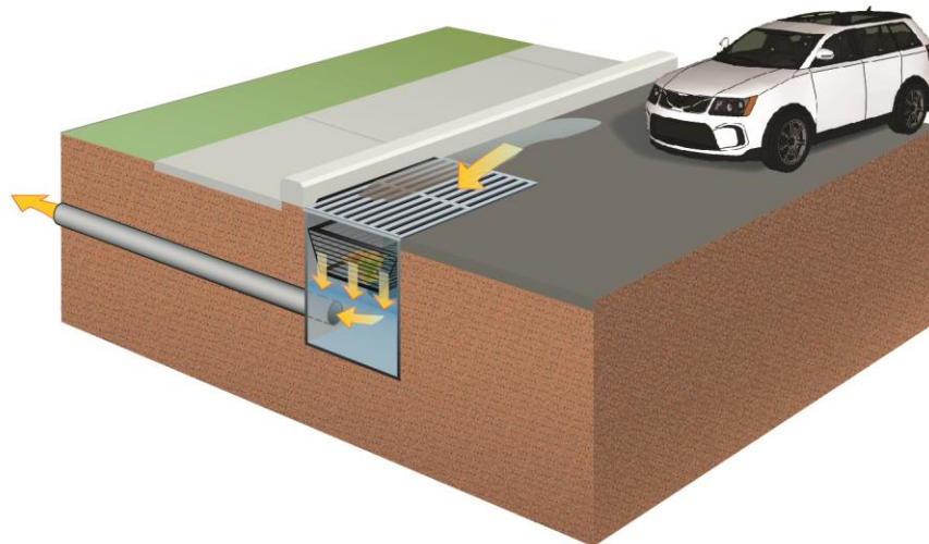
Figure B1-9. Typical distributed source control structural BMP (arrows indicate water pathways).
