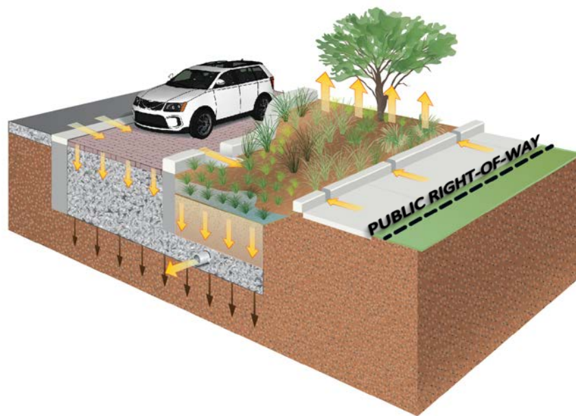
Figure B1-4. Typical distributed green street schematic (arrows indicate water pathways).
