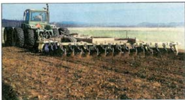
A second pass over the field with the tandem disk at a 45 to 90 angle to the first disking assures more complete incorporation of the ash. Photo by University of California
