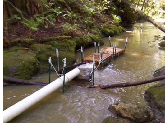
This is a smolt trap. On the South Fork of Freshwater Creek, Fish and Game maintains this trap. Photo by Matthew Buffleben
