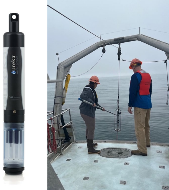
Figure 6. Eureka Manta+35 CTD: On the left is a Eureka Manta+35 CTD which measures conductivity (salinity), temperature, depth, pH, dissolved oxygen, and turbidity. On the right is an image depicting deployment/retrieval of a Eureka Manta+35.
