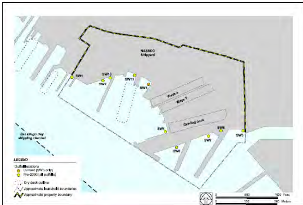
Figure 11-2 Storm Drain Outfalls at NASSCO's Leasehold
