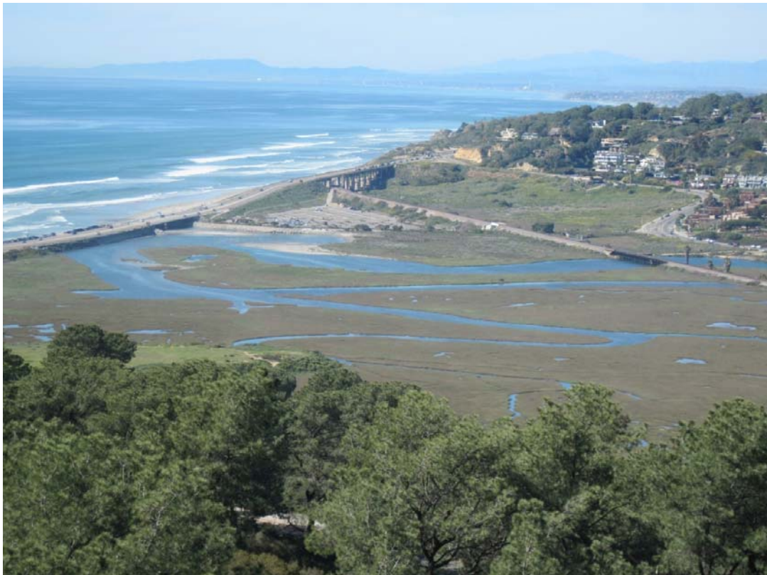
Figure 6. Photograph of Los Peñasquitos Lagoon. Tidal flows enter the Lagoon via a channel beneath the U.S. Highway 101 bridge and then bifurcate into the eastern and western branches.
