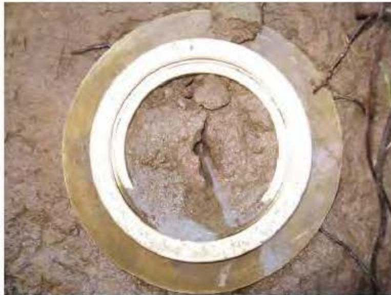
Hole created in cohesive bank material by jet impinging on surface
