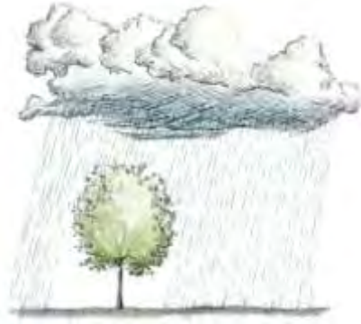
Figure 2-1. Vegetation reduces runoff by intercepting a portion of the total rainfall and preventing water from entering the drainage system. (Illustration by Jennifer Natali).
