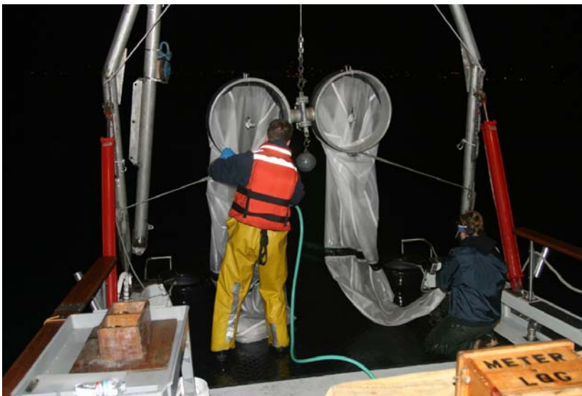
Figure 2. Night sampling for larvae using a bongo net. In this image the net has been retrieved after being towed and is being rinsed to ensure all contents are moved down towards the cod end for sorting and analysis.
