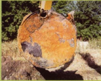
Removed formerly leaking and corroded UST.
