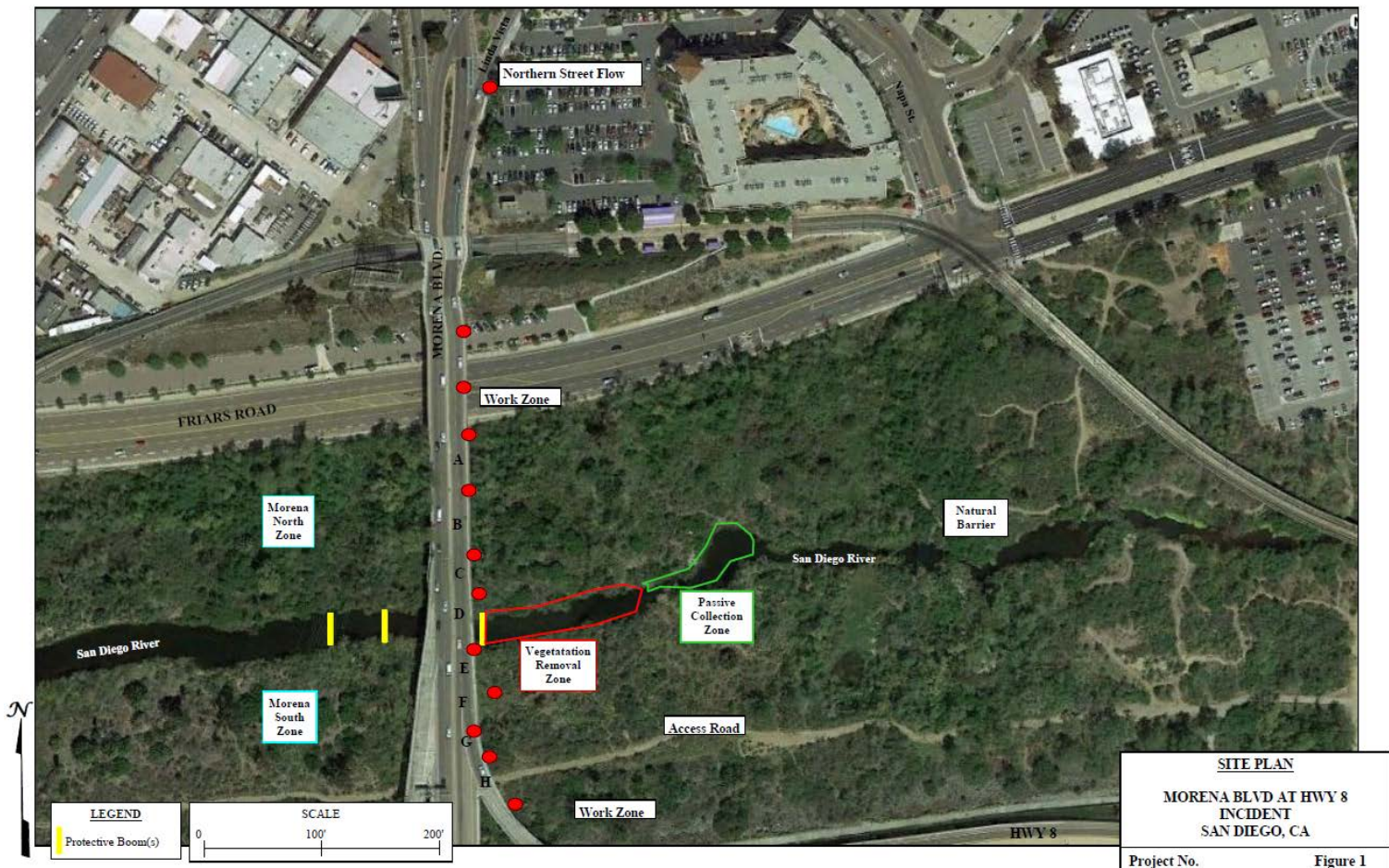
Figure 1: Ariel view of the spill site. Red dots indicate locations of drain ports on bridge.
