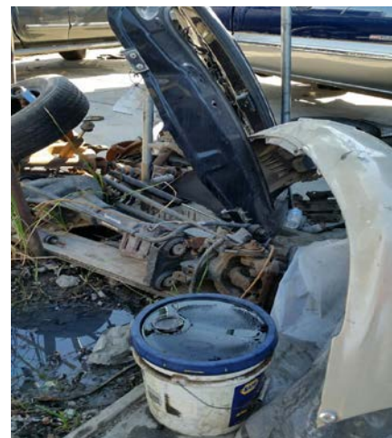
Dismantled car parts leaking fluid to ground, and improperly stored waste.
