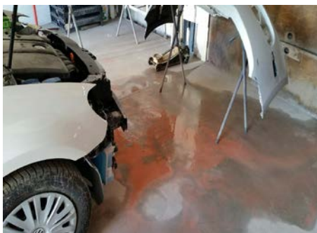
Engine fluid carelessly drained to the floor raising potential for discharge to reach ground or the storm drain.
