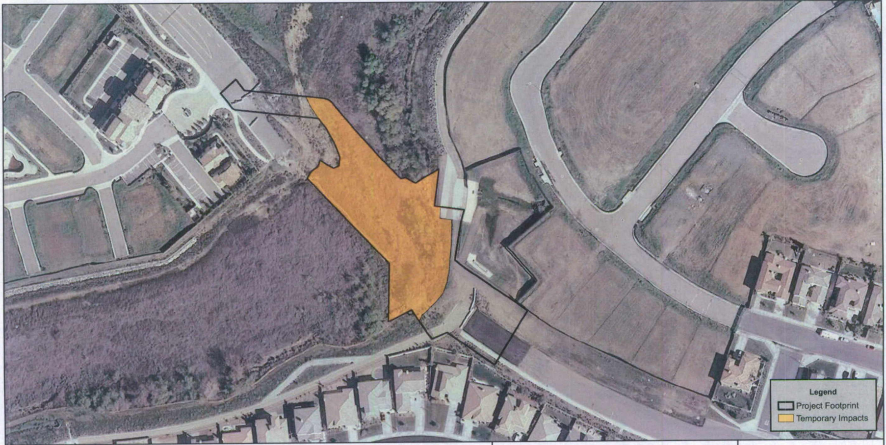
Figure 5b Proposed Temporary Project Impacts French Valley Creek Slope Protection at Skyview Road and Water Supply Crossing
