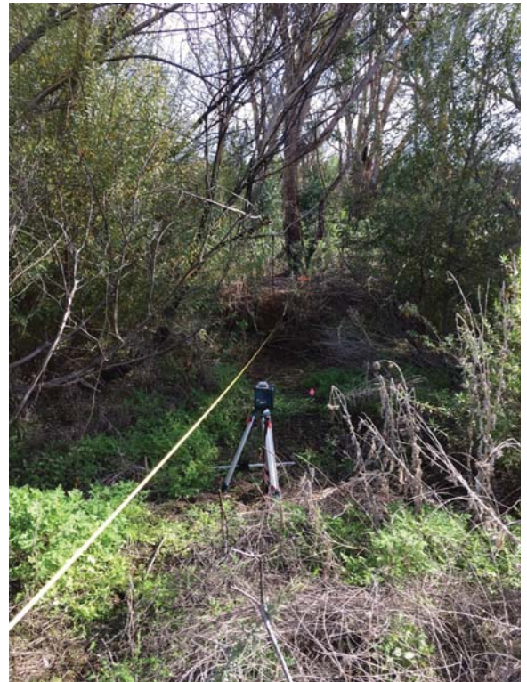
Figure 5. View looking southeast showing cross section XS3 with the surveying level moved to the turn point location and turn-point benchmark visible (pin flag location).
