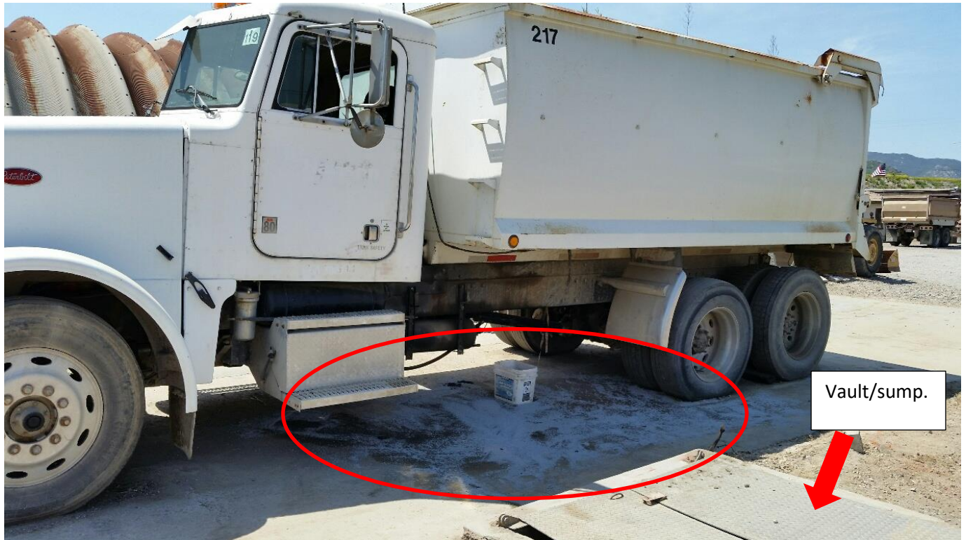
Photo #42- Large quantity of absorbent under truck. Note close proximity to vault/sump.
