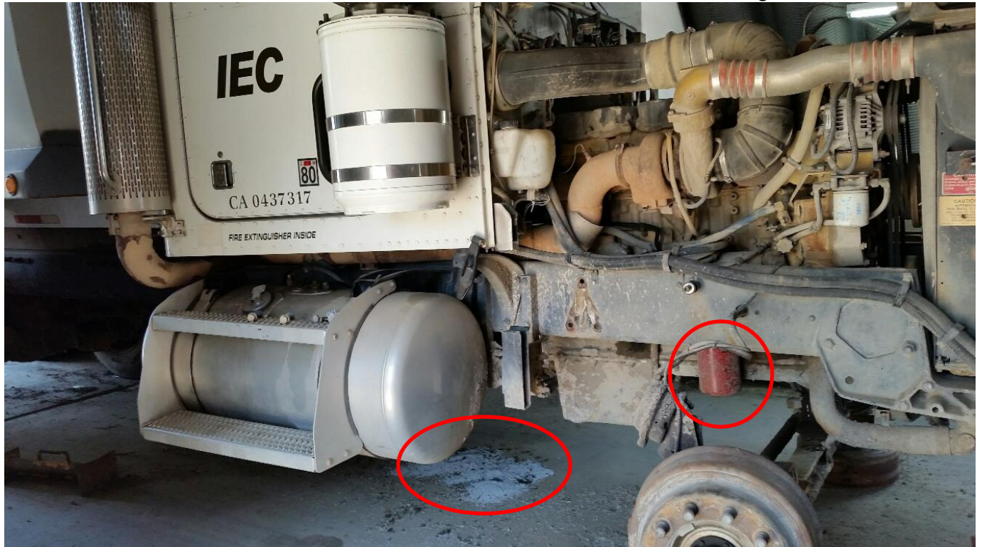
Photo #21- Absorbent on spilled/leaked oil under IEC truck that appears to be in servicing/maintenance. Drip pans should be used. Note red oil filter on the truck.
