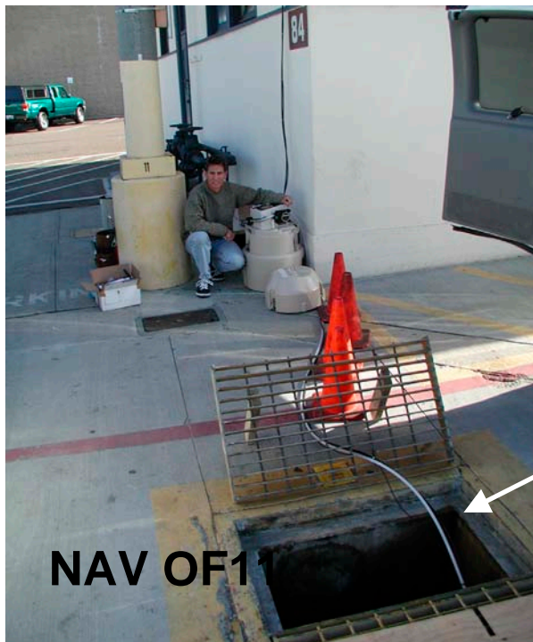
Figure 8. Naval Station San Diego storm water monitoring location for outfall 11. The rain gauge was placed on top of Building 84 in the background. The solar power panel and RF link were attached to the light pole next to the building. The short distance between the building and the grate was secured by traffic cones to protect the sample line and cabling. The inset at the right shows plywood covering the catch basin when the Graving Dock was active.
