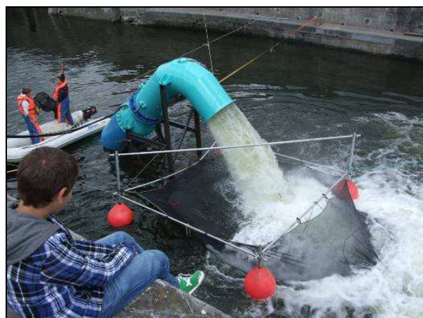
figure 2.2 Forced exposure of fish to the running pump.
