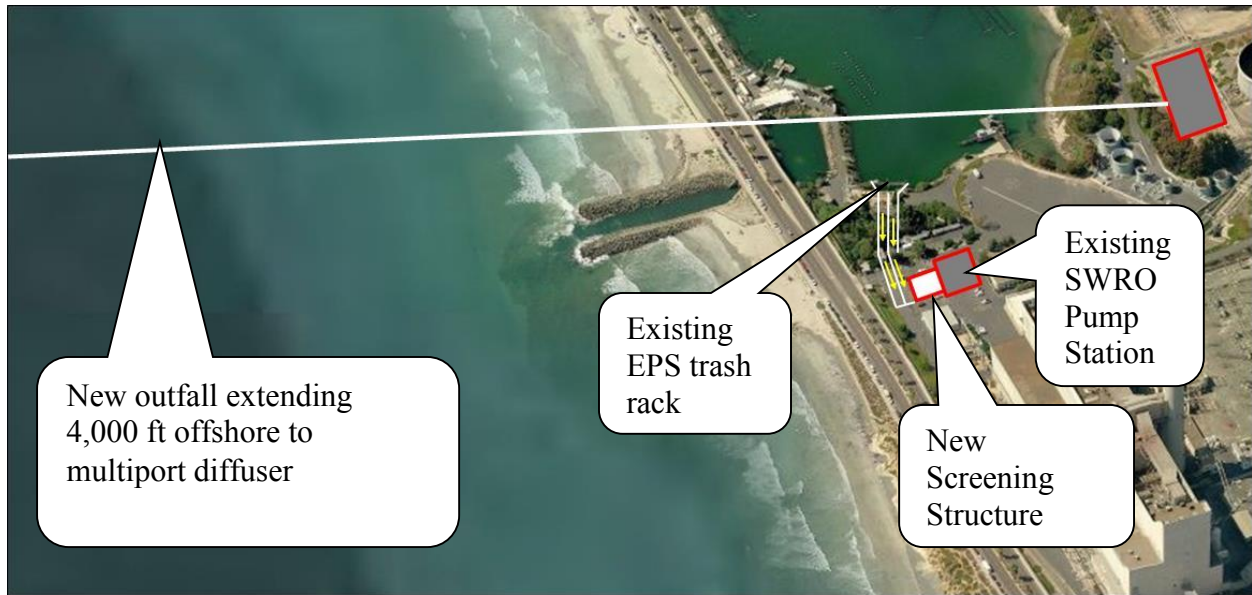
Figure 22. General schematic of the layout of the CDP with a screened intake and discharge diffuser.
