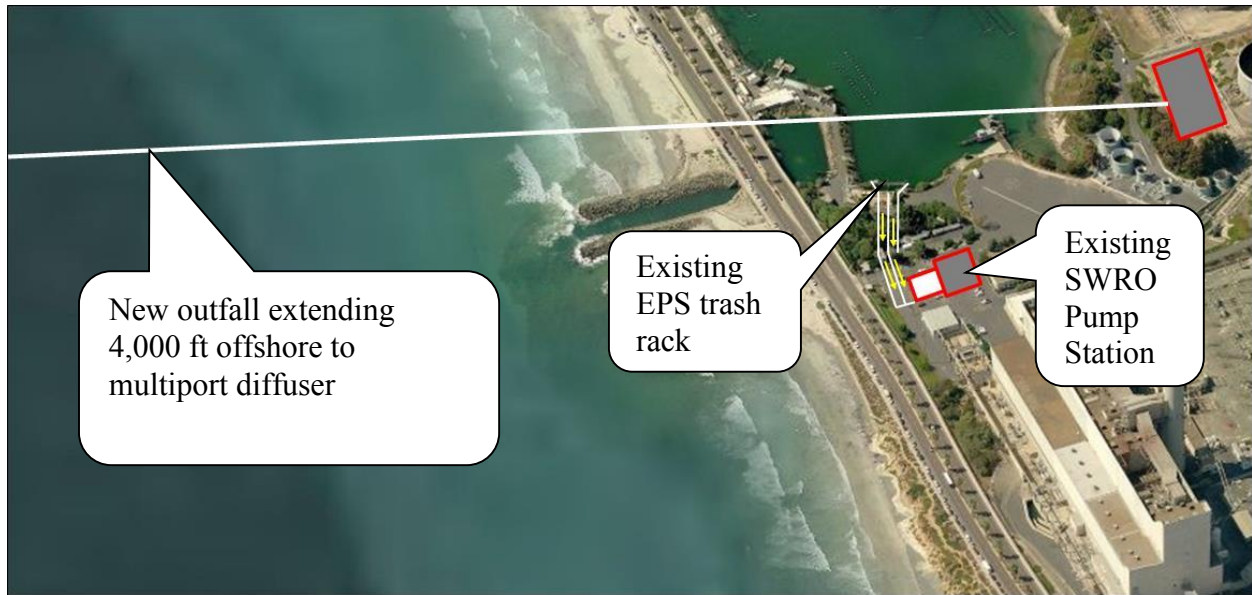
Figure 6. General schematic of the layout of the CDP with a screened intake and discharge diffuser.
