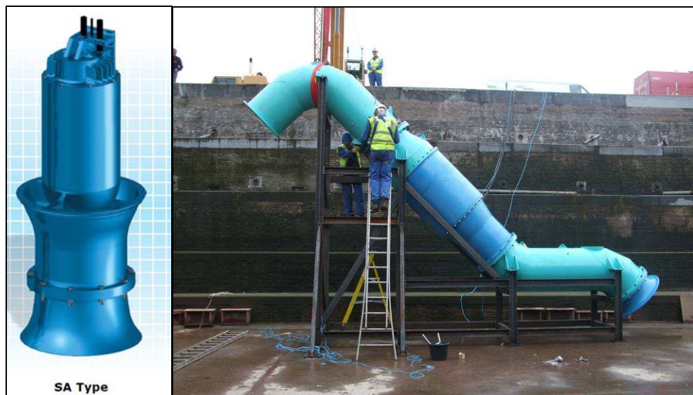
figure 1.1 Drawing (left) and picture (right) of Bedford Pumps submersible axial pump SAF.90.05.12. Right: the pump with in- and outlet pipes, mounted on the rig.
