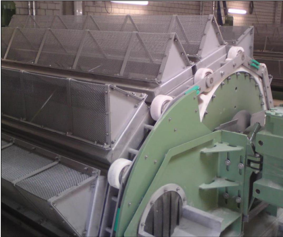
Figure 16. Example of BWT center-flow traveling screen panel mesh (courtesy Bilfinger Water Technologies).
