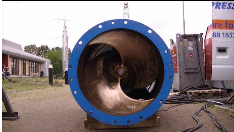
figure 1.2 Impeller of Bedford Pumps SAF.90.05.12 pump.
