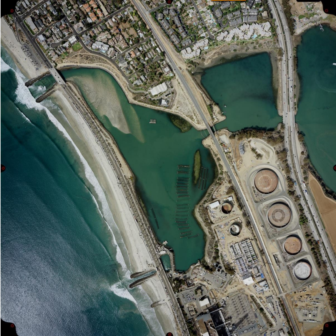
Figure 1: Aerial view showing spatial relationship between the discharge pond located in the southwest corner of the Agua Hedionda Lagoon immediately east of Carlsbad Blvd. and the discharge channel bounded by a pair of jetties that terminate in the surf zone. (photo courtesy of NRG Energy).
