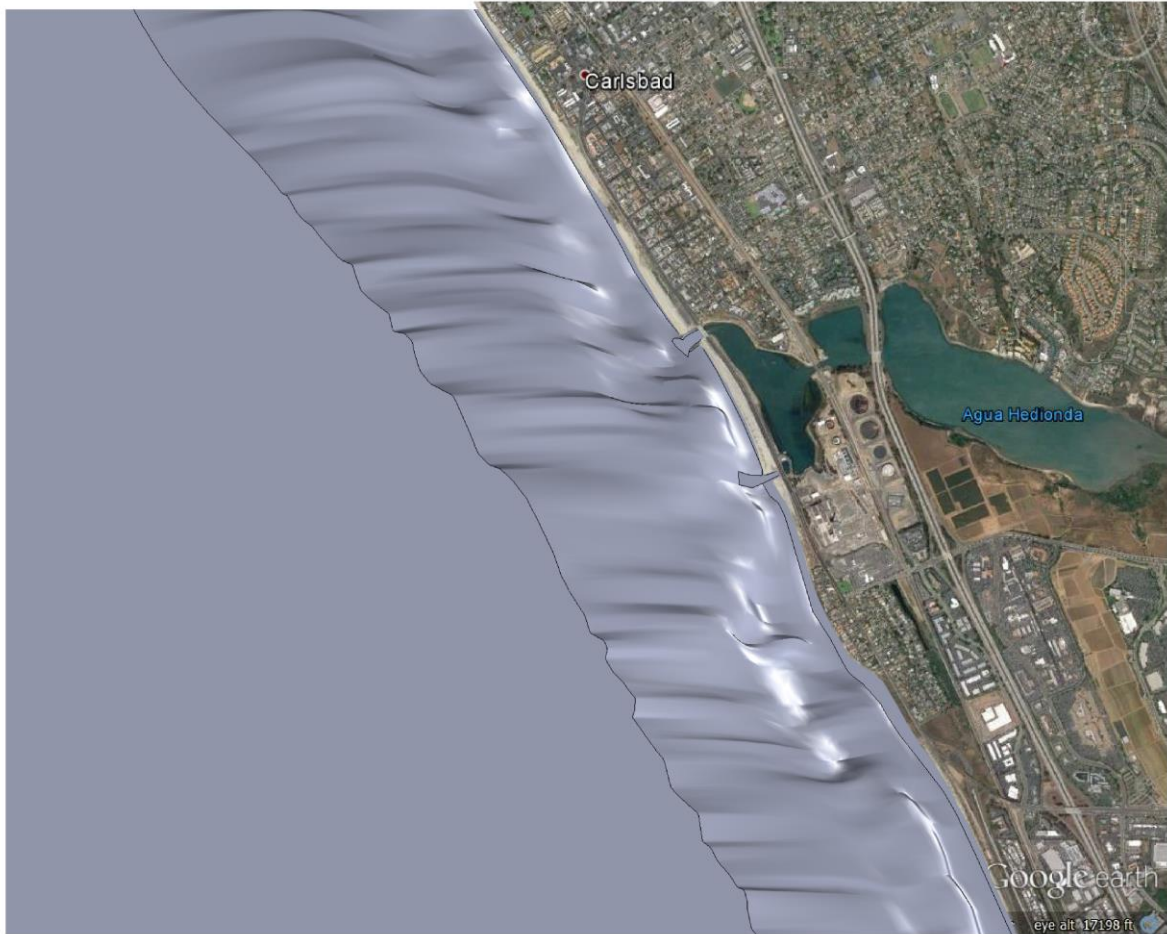
Figure 3: Three-dimensional CAD bathymetry creating a farfield computational grid at 0.1 arc-second horizontal resolution and covering an area of receiving water 6 km x 6 km in the vicinity of Agua Hedionda Lagoon. Intersection of trapping level with the seabed shown as black offshore contour
