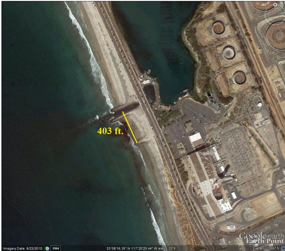
Figure 5: Google Earth image of the South Beach Groin presently located 403 ft south of the cooling water discharge channel at Encina Power Station, Carlsbad, CA.
