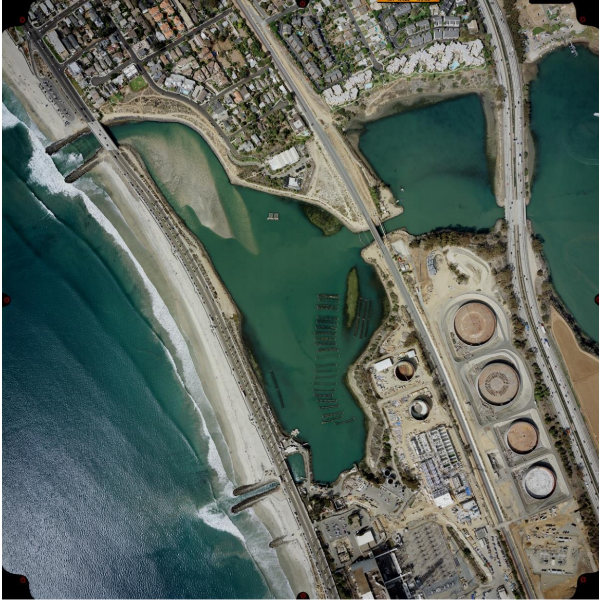
Figure 2: Aerial view showing spatial relationship between the ends of the discharge jetties and the surf zone. (photo courtesy of NRG Energy).
