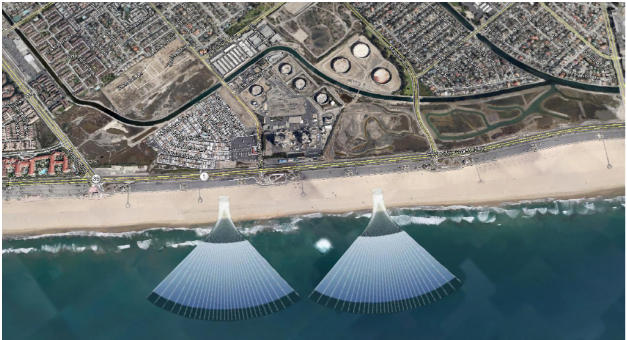
Figure 3.5. Conceptual diagram of the HDD wells at Huntington Beach (from Neodren, 2014).
