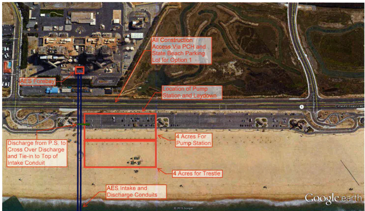
Figure 3.11 Location of Onshore Pumping Station Facilities
