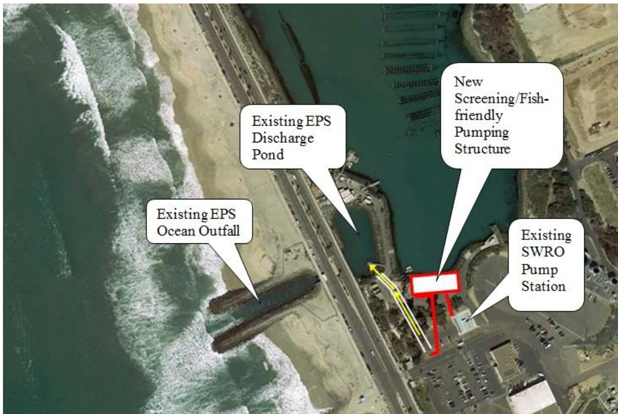
Figure 2. General layout of the CDP with Lagoon shoreline location of the New Screening/Fish-friendly Pumping Structure.
