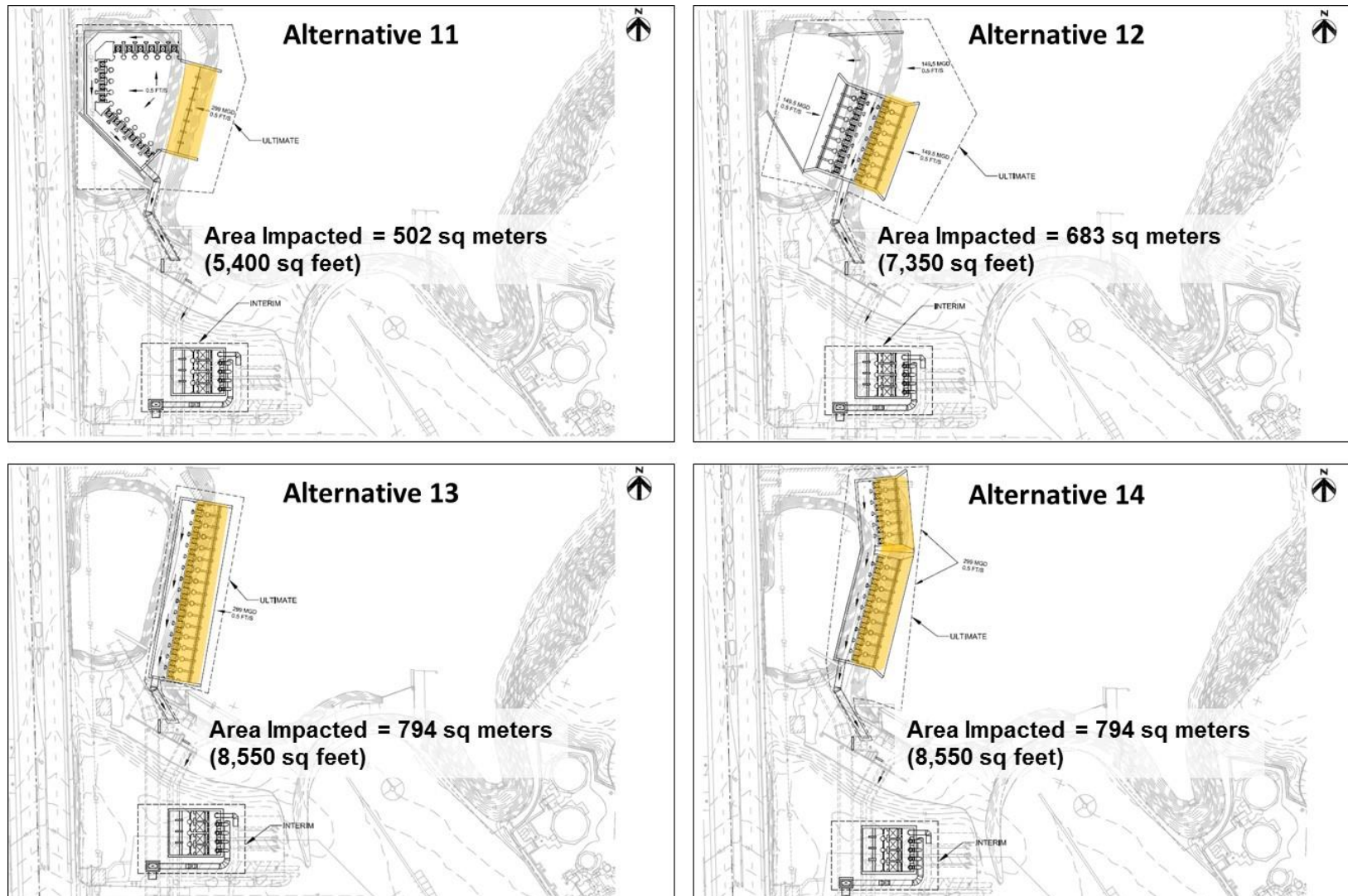
Figure 3. Estimated footprints (in orange boxes) for the four conceptual designs for the Lagoon shoreline intake system for the CDP.
