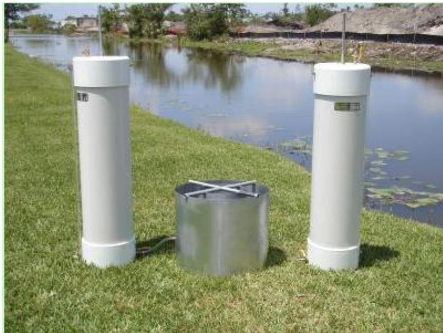
Figure VII.10. Double Ring Infiltrometer Set-up with Mariotte Tubes
