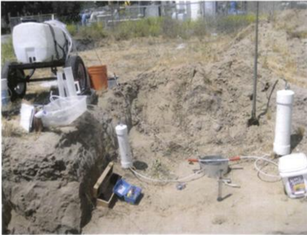
Figure VII.11. Double Ring Infiltrometer Set-up for Test at Basin Surface Elevation
