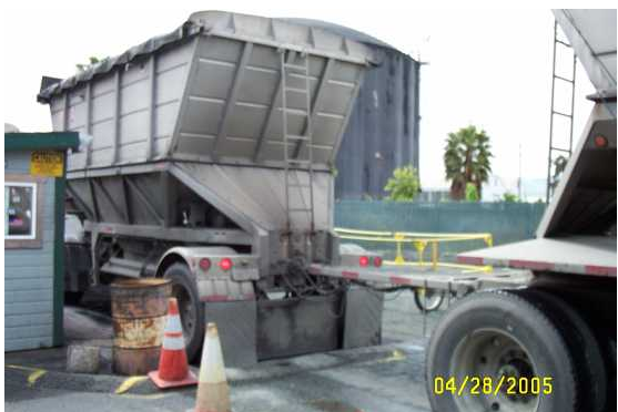
Bottom loading truck depositing coke to underground conveyor
