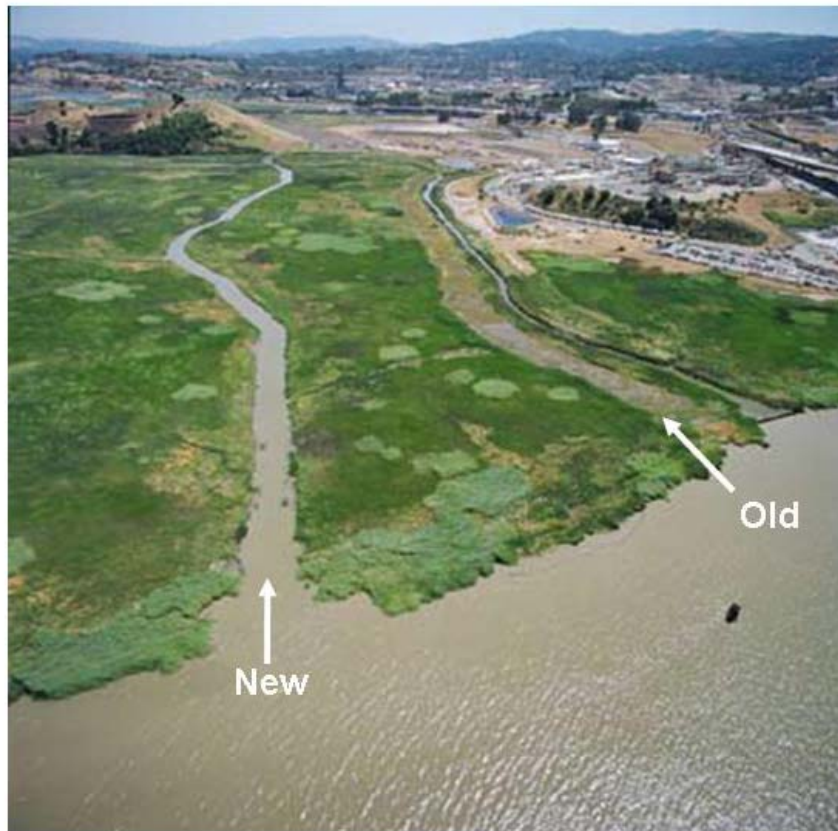
July 2006 aerial photo of the new Peyton Slough alignment with partial revegetation of the capped, old alignment.
