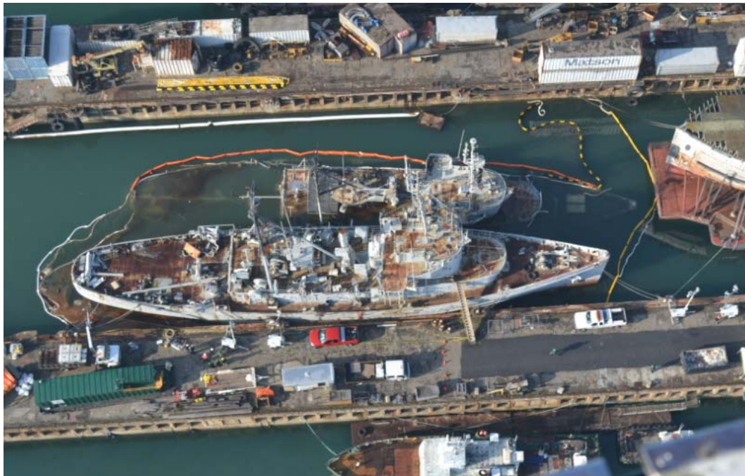
Photograph 2. Aerial view of the sunken Tiger Tug and some of the booms used to contain materials discharged from the vessel. Additional booms and containment equipment, such as pumps, were used to minimize any harm to the Bay.
