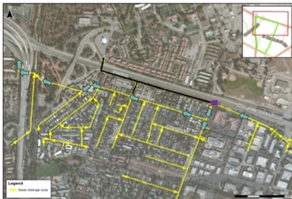
Figure 4c. Sanitary sewer pipeline locations prior to 1966 in vicinity of TCE hot spots.
