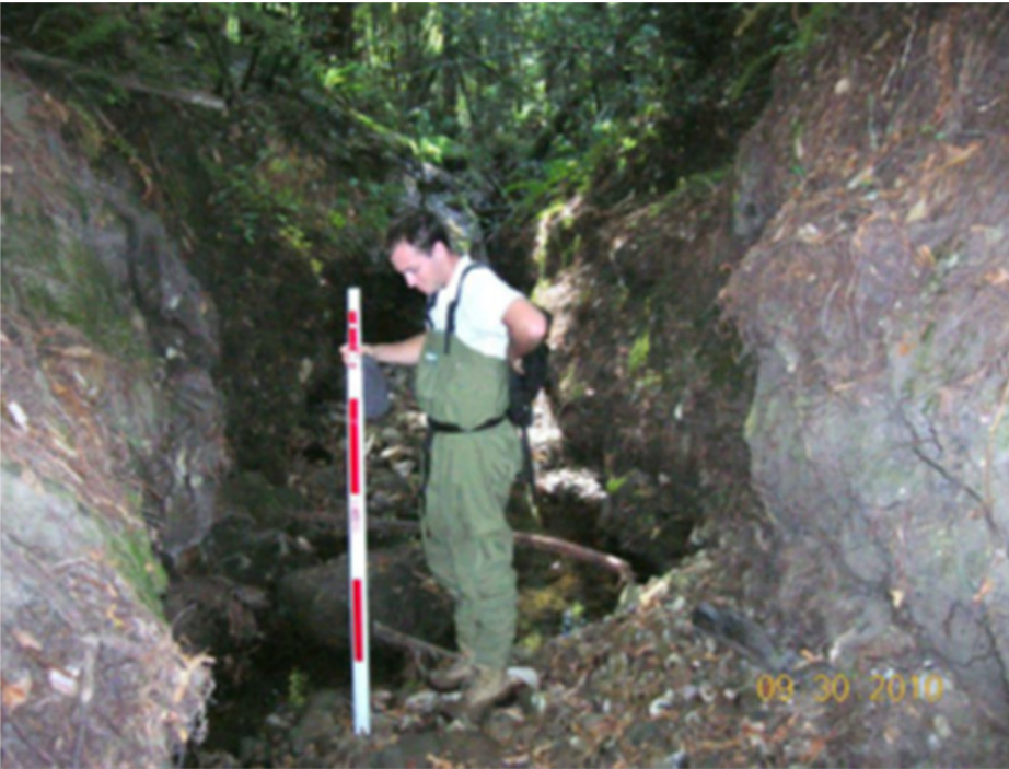
Figure 2a. Water Board staff measuring stream incision in Pescadero Creek.
