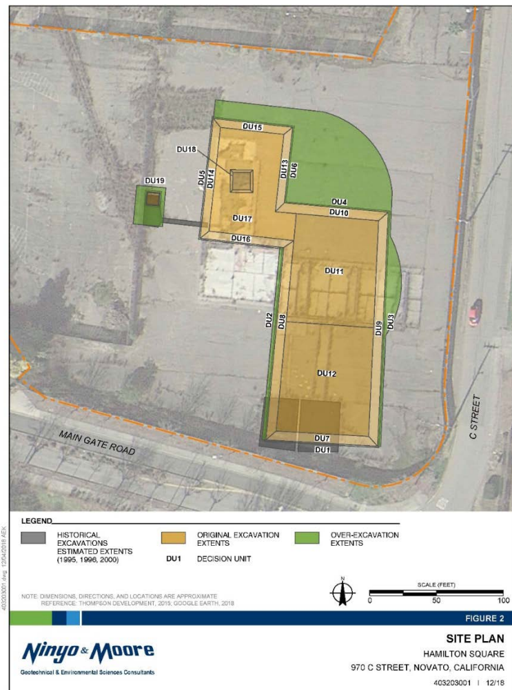
Figure 3 – Footprint of historic gas station, soil excavation footprint, and planned redevelopment footprint with Decision Units (DU)
