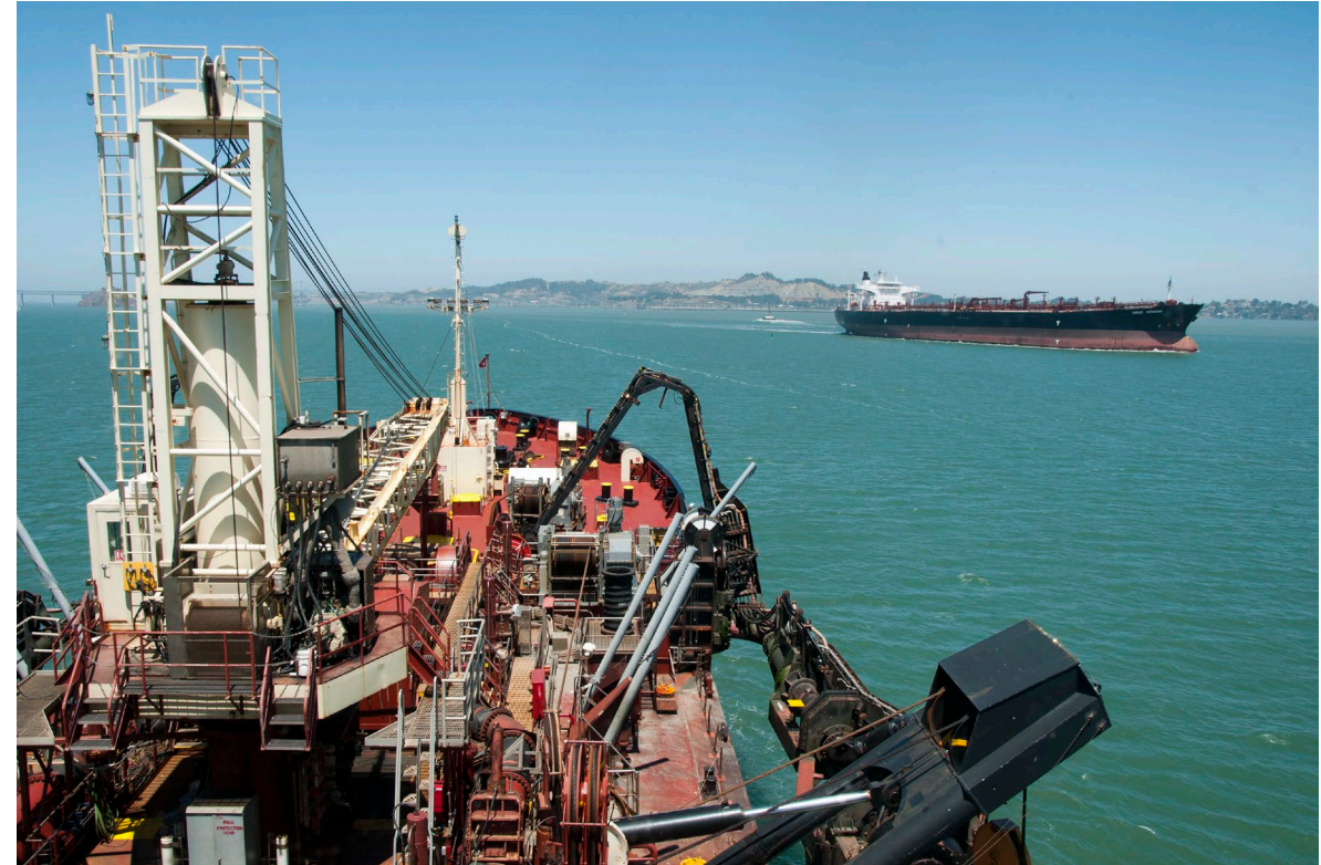
Photo of a hopper dredger contracted by the USACE San Francisco District to dredge various locations around the San Francisco Bay.
