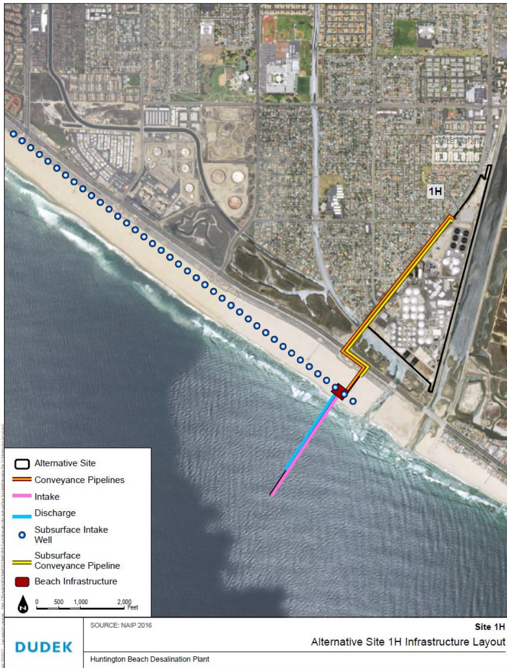
Figure 11. Alternative Site 1H Location and a Conceptual Plan for Surface and Subsurface Intakes
