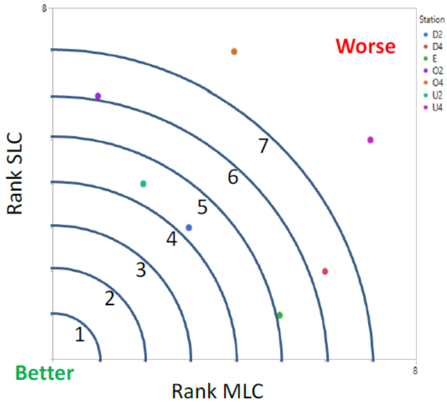
Figure 14. Use of Euclidean distances to assess joint metrics of impact. Arcs indicate distance from the origin (Source: Raimondi 2019).
