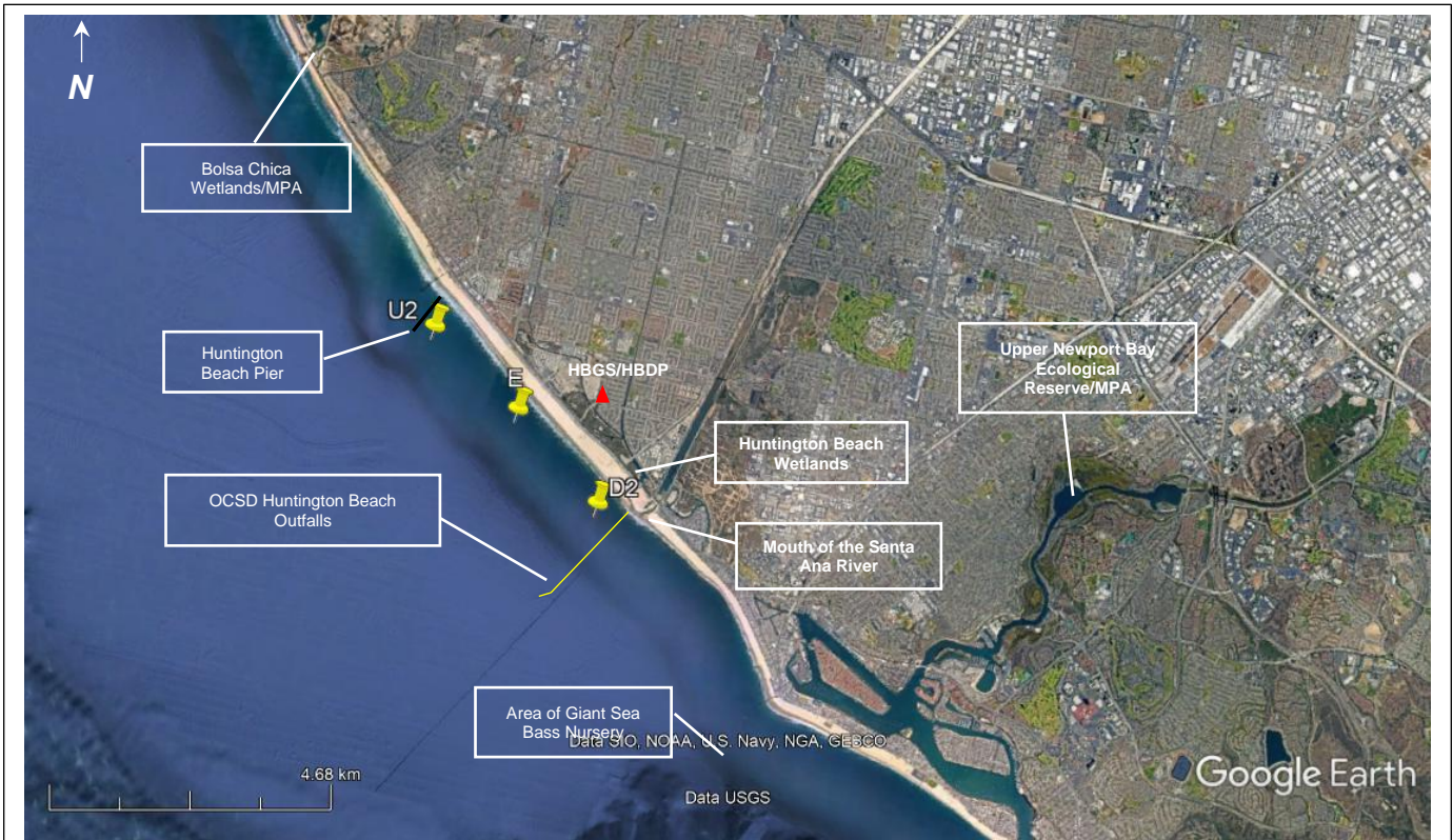
Figure 17. Locations of the proposed surface intake (Station E) and the two alternative stations (Stations D2 and U2) and their proximity to local wetlands, the mouth of the Santa Ana River, the OCSD outfalls and the Huntington Beach pier. (Source: Santa Ana Water Board staff image)
