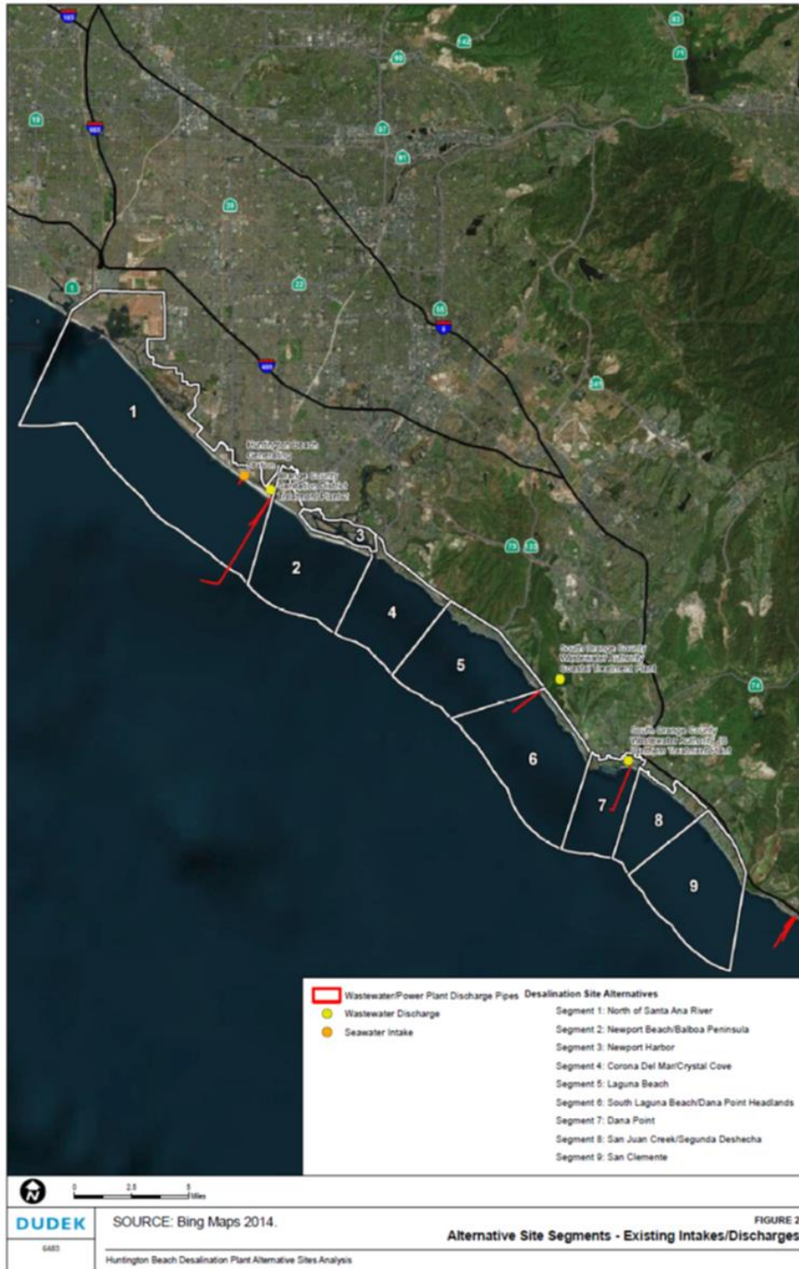
Figure 5. Existing Intake and Discharges located within the Nine (9) Segments Evaluated (Source: Discharger’s Appendix E, Figure 2)
