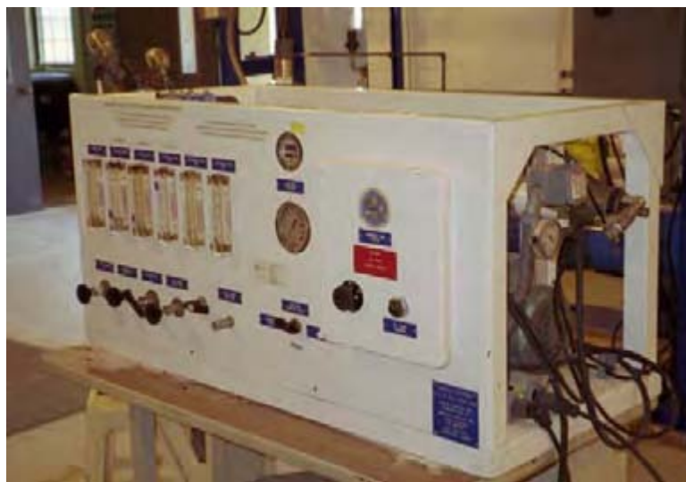
FIGURE F4 Single Element Unit Equipped with Zeta Rod Used during the EDR Recovery Testing
